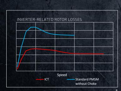
In addition to the remarkable increase in field weakening capability, the innovative "Integrated Choke Technology" leads to a significant reduction in rotor losses caused by the inverter. As a result, the rotor temperature is significantly reduced. This reduction has a positive effect on the thermal load on the magnets, shaft and bearings, which in turn leads to a significant increase in service life.
