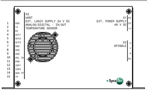
5.3 Power Supply Connection X1 (Connector TBP01P1-508-03BE)
