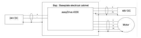
The devices must not be connected directly to low voltage supply networks. If the devices are to be connected to a low-voltage supply network, appropriate interference suppression measures must be taken.
