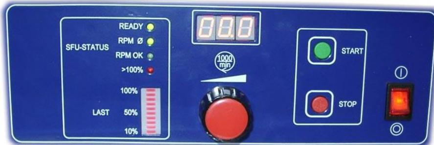
With the **START** **STOP** -key the spindle is started and stopped. The rotational speed is adjusted with the radio knob. The actual rotational speed is displayed on a 3digit LED.
