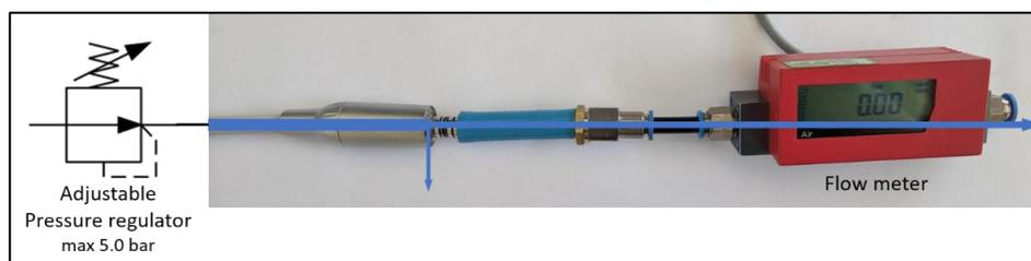
The handpiece cooling air is set with an adjustable pressure regulator as follows:
