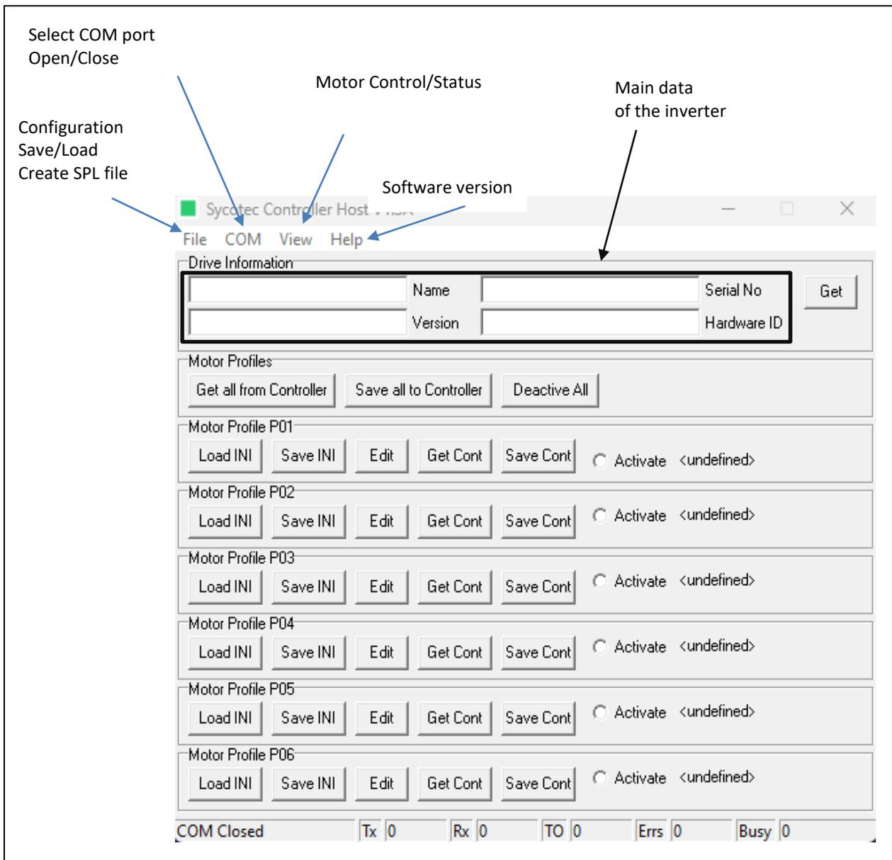
On the **start page**, the main data of the inverter are displayed when one is connected to the inverter and presses the "Get" key. In addition, the motor profiles can be selected and activated. The profile selection is described in Chapter 5.1.3.
