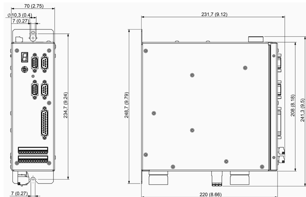
Fig. 4: Dimensions 0362x40EF (480 V mains supply) in mm (inch)
