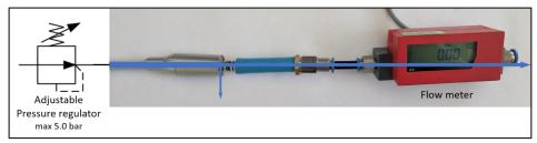
The handpiece cooling air is set with an adjustable pressure regulator as follows:
