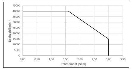
The characteristic curve may vary depending on motor control and power supply used.
