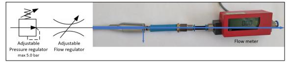
The handpiece cooling air is set with a pressure regulator and an adjustable restrictor as follows:
